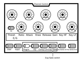
Expander/gate parameters in Channel Control
