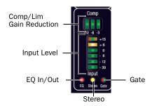
Input channel meters and LEDs
