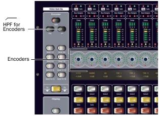
HPF controls for Input Channels
