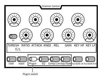
Plug-in switch in Channel Control
