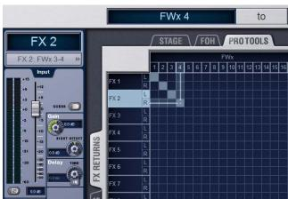
Patching FWx channels to FX Returns for playback
