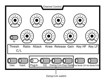
Compressor/limiter parameters in Channel Control
