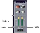
Selected Channel meters and LEDs
