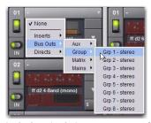
Assigning plug-in Input source to a Group bus
