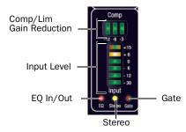
Input channel meters and LEDs
