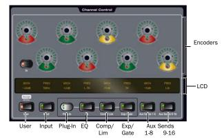
Channel Control encoders, LCD and mode switches
