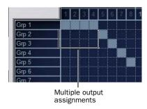
An Output bus assigned to multiple hardware outputs
