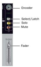
In its default Selected Channel mode the Flex Channel mirrors the currently selected channel. The Flex Channel encoder follows the current Encoder Assignment mode (gain, pan, HPF, or a send). The Flex Channel LCD shows the current channel name.
