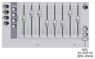
Input fader banking and assignment switches
