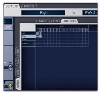
Routing the Mains bus to FWx channels for recording
