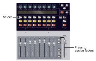
Bank switches for Output channels
