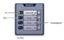
LED indication of in circuit and out of circuit (bypassed) inserts
