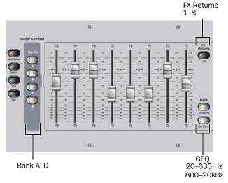
Input fader banking and assignment switches
