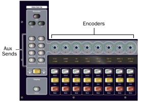
Encoder assignment switches for input channels
