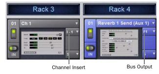
A mono plug-in inserted on a channel (at left) and a stereo plug-in assigned as a bus processor (at right)
