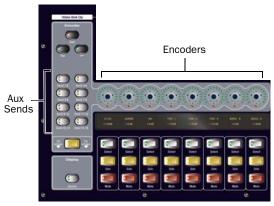
Encoder assignment switches for input channels
