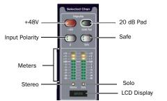
Selected Channel Input controls, meters and displays
