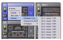
Assigning a channel Direct Out as a plug-in input source in the Plug-Ins
