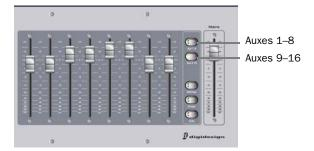
Auxes switches in the Output section
