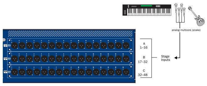
Figure 4. SC48 I/O slots A-C for stage inputs 1-48
