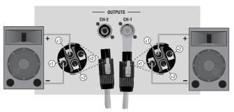
Figure 3.5 Speakon Output Connector Wiring
