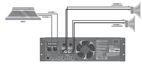
Figure 3.8 System Wiring, Stereo Mode
