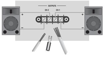
Figure 3.6 Barrier Block Output Connector Wiring
