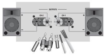
Figure 3.7 Binding Post Output Connector Wiring
