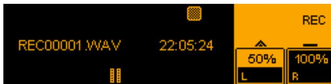
**i** The time display on the display panel indicates the remaining recording time left on the storage device.
