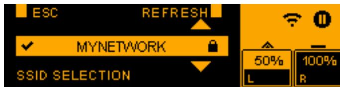
The available networks are then shown on the display panel. Encrypted networks are marked with a lock icon.
