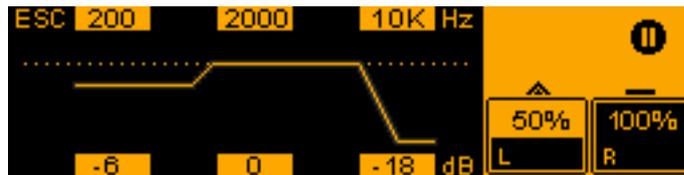
▶ Configure the master EQ using the jog dials that are assigned the following functions:
