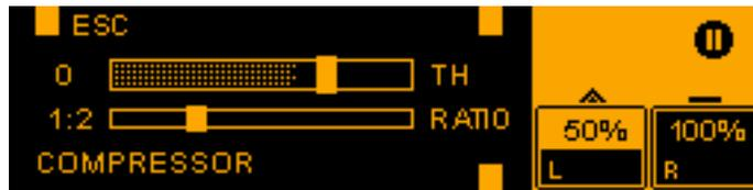
**i** The dotted area in the **TH** slider displays the level of the audio signal.
