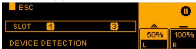
The device detection process is performed and the display panel displays the slots in which a device with media control protocol has been detected.
