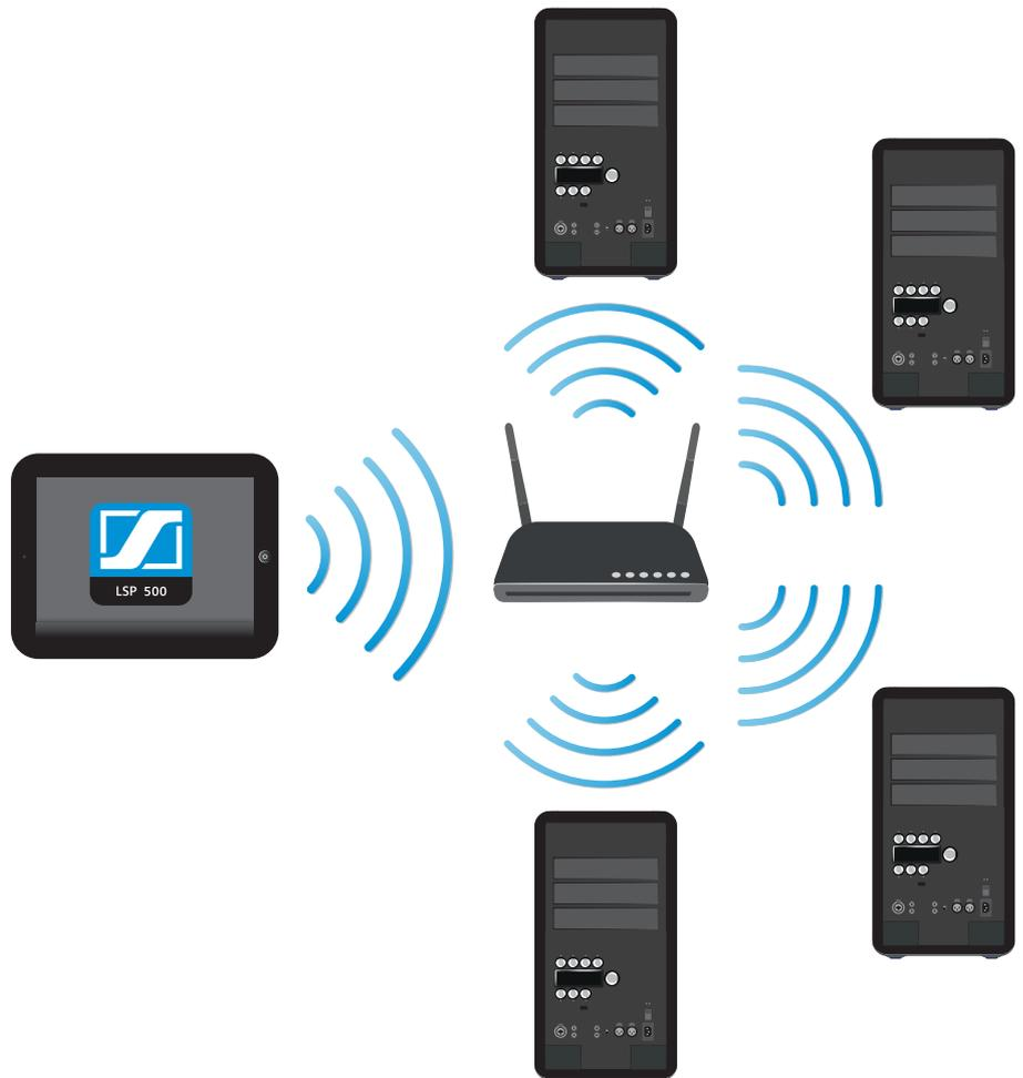
**i** In order to be able to operate the LSP 500 PRO from your tablet using the app, you first have to connect the LSP 500 PRO to a wireless network (WLAN). For information on how to connect the LSP 500 PRO to a wireless network, refer to page 42.
