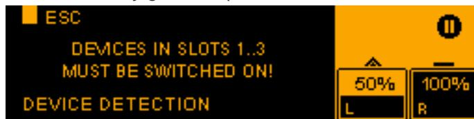
▶ Switch the installed ew devices on before starting the device detection process.
