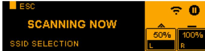
When opening this menu item for the first time, a scan for available wireless networks is run. **SCANNING NOW** appears on the display panel and the WLAN icon flashes in the status area.
