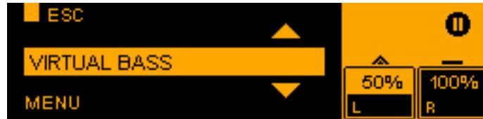
The opened menu level or menu item is shown at the bottom left of the display panel. The **ESC** function allows you to return to the previous menu level.
