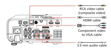
**Note:** If you are connecting a streaming device, you can also connect it to the projector's **USB-A** (flat) port for power.
