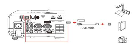
If you connect a digital camera, USB flash drive, or USB storage device, you can use the projector's PC Free feature. You can also connect other Epson document cameras to the projector. See the online *User's Guide* for details.
